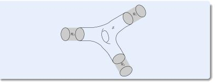
Particles are non-interacting in the ends but may be interacting in the compact region S (electronics, photonics, spintronics, ....)
